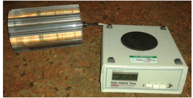
Figure 4. Electrometer RAD-CHECK connected to the ionization chamber.
