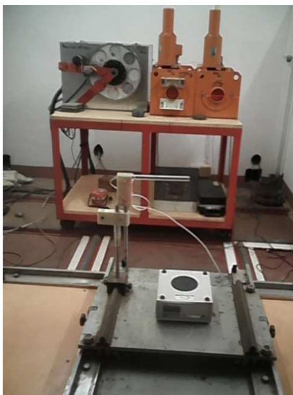
Figure 3. Experimental device for the irradiation of the reference instrument in the SSDL-Madagascar.
