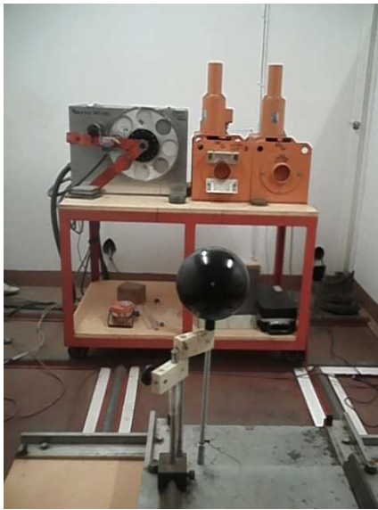
Figure 2. Experimental device for the irradiation of the reference instrument in the SSDL-Madagascar.
